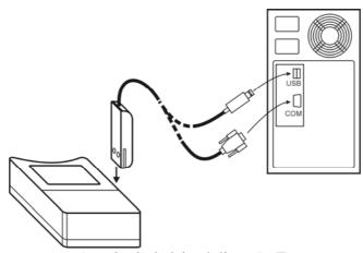
communication adapter is necessary (not included in delivery). For connection via RS232 serial
