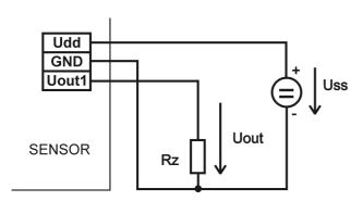
$\label{eq:maximum load current of each voltage output} \ is \ 0.5 \ mA$
