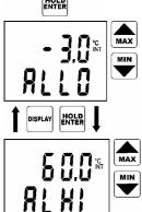
Reading ALLO indicates adjusted lower alarm limit (here air temperature). Set the desired value by means of the arrow keys. Press and hold the arrow key UP to make value increase fast. Press and hold the arrow key DOWN to make value decrease fast. Release the arrow key and press ENTER to confirm new limit.
