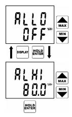
Then you are offered to set alarm of other input value (here relative humidity). The procedure is the same as the above temperature limit setting. Alarm activation of each value can be disabled by setting lower alarm limit of the desired value up to its maximum. This is indicated by OFF reading at the position of numeric value. Value of upper limit of the same alarm is indifferent.
