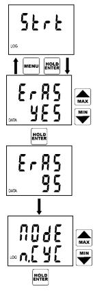
If it is needed to clear the memory before logging start, first it is necessary to select menu item logging START (symbol Strt) and confirm by pressing ENTER key.
