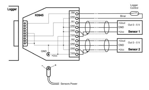
At this case sensor is possible to power e.g. from ac/dc adapter, connected via coaxial power connector to K0945 adapter. Supply voltage and the power of the applied ac/dc adapter depend on type of connected sensor.
