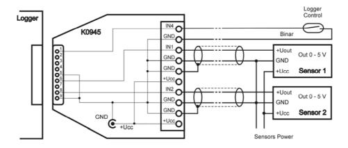
Connection to sensor signal. Power supply is located near the logger:
