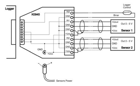
At this case sensors are possible to be powered e.g. from ac/dc adapter, connected via coaxial power connector to K0945 adapter. Supply voltage and the power of the applied ac/dc adapter depend on type of connected sensors.
