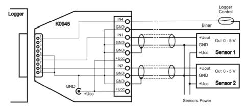
Connection to sensor signals. Power supply is located near the logger:
