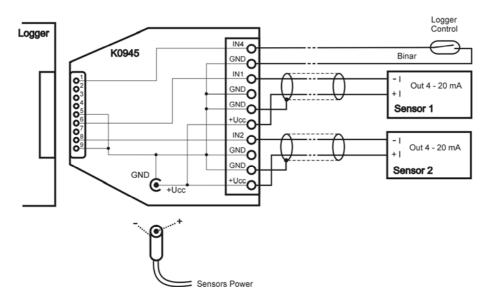
In this case it is possible to power current loop e.g. from ac/dc adapter, connected via coaxial power connector to adapter K0945. Power voltage level depends on applied transducer type.
