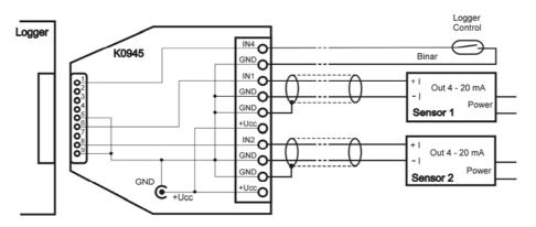
Logger connection to transducer requiring powering of current loop by external source
