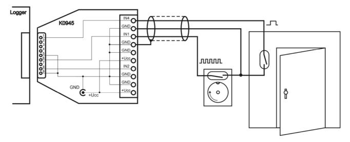
Let co-axial power connector of the K0945 adapter not connected, there is no need to supply the adapter. Monitored devices in the figure are only for illustration.
